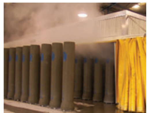
Steam chamber for concrete pipes
