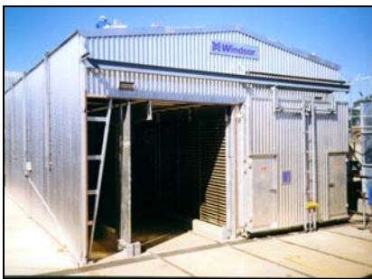
Double track kilns
